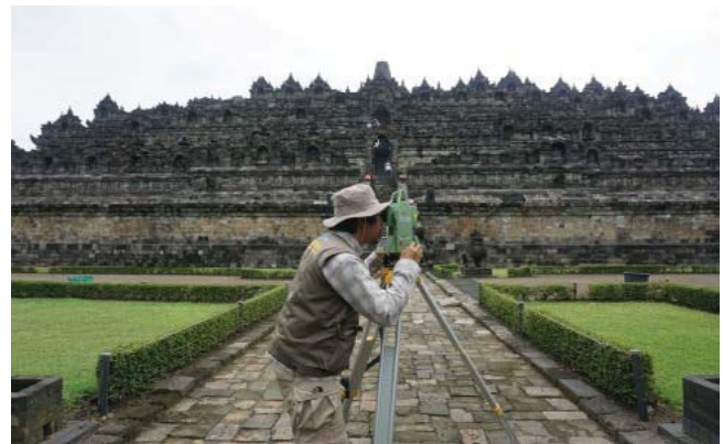
Gambar II.3. pengukuran 3D Laser scanning dan Total Station
